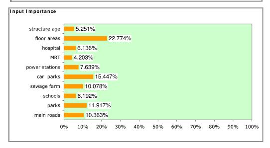
However, a drawback of ANN can be observed in the above graph of the inputs' relative importance: no signs are attached the calculated weights. Thus the interpretation of the relative weight requires the simultaneous running of a multiple regression. The task is not a major imposition on the analyst since - the ANN program used here being Excel based - it takes only a few more clicks to generate the regression results summarised below.
