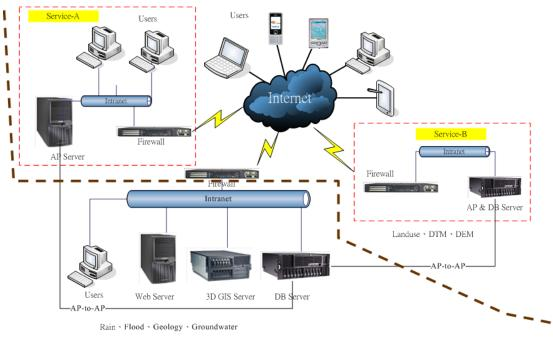
Figure 7. Software and hardware structure platform
