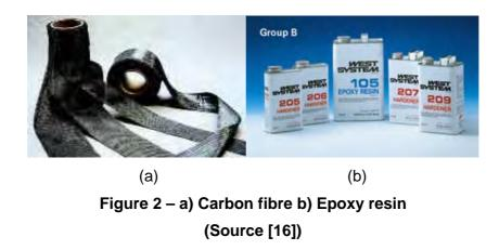
The fundamental building block of fibre composites is the *laminate*. The *laminate* consists of a number of layers of reinforcing fibre stacked in a preset pattern and bound by a hardened resin. The strength and stiffness of the laminate depends largely on the amount of fibres and the direction which the fibres are laid. Laminates which are very strong in one direction can be made by aligning the fibres in all layers in the same orientation.
