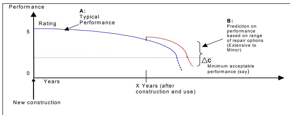
Figure 2 Typical deterioration trend of building element
