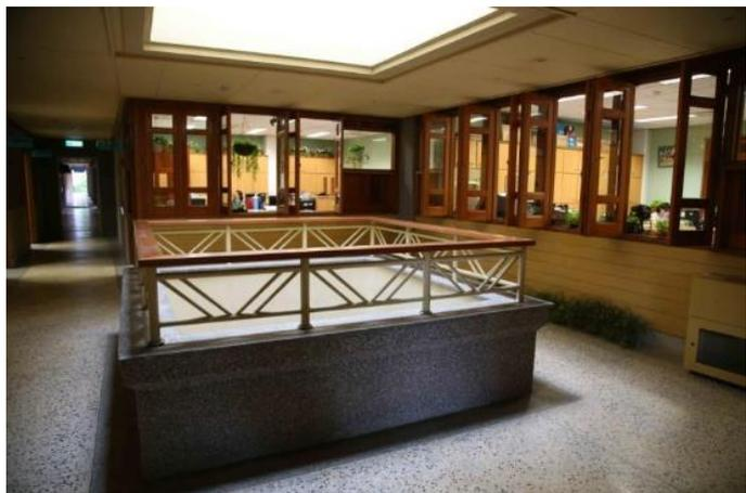
In addition, there is a nature pool area located on the west side of the building that help to cool down the area during hot summer afternoon (Figure 16). In addition, part of the pool is extended inside the building that further improve the cooling effect (Figure 17).
