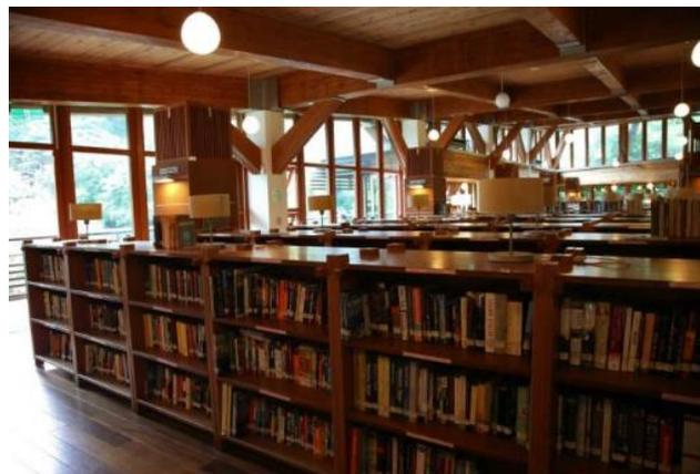
The thoughtful design of a central atrium with large windows is to save energy as the large amount of windows allow natural light to substitute interior lighting (Figure 5), and north-south direction openable windows provide cross-ventilation that reduces the need for fans and air-conditioning (Figure 6).
