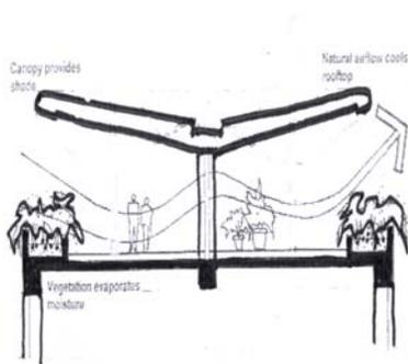
**Roof insulation** - The flat roof is constructed of 100mm thick reinforced concrete with 50mm thick polystyrene insulation. A secondary roof was provided to further shade part of the insulated roof and this provides spaces at the rooftop for the office activities. The roof is surrounded by planter box which also acts as the safety railing. Rainwater from the secondary roof is harvested for watering the plants. By not having a green roof at the top the designer has reduced the maintenance cost.
