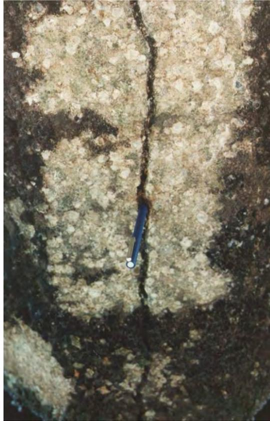
**Figure 9 – Typical longitudinal crack in concrete due to alkali / silica reaction
